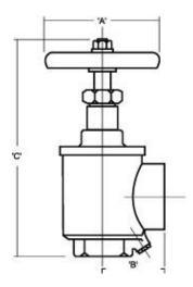
A= 4" (100mm) B= 2 1/4" (56mm) C= 8" (OPEN) (200mm) C= 7" (CLOSED) ((175mm) Weight: 4lbs 1.8Kg Working Pressure: 300 lb (2070 Kpa)
